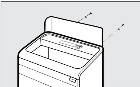
2. Slide 1 screw cover cap on each of the self-taping screws, then use 2 of the screw assemblies to attach signage to back panel of container base.
