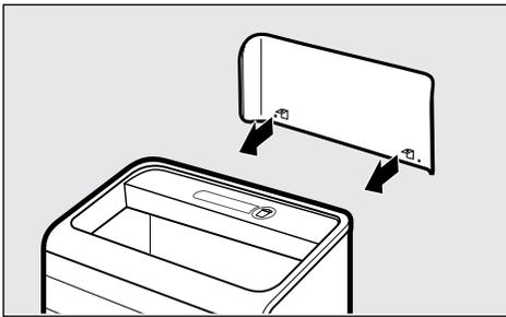
1. Slide additional signage into back of container; signage tabs should fit in the gap between the lid and base.
