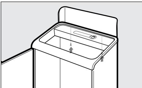
3. With lid attached to container, insert remaining 2 self-tapping screw assemblies through the aligned tabs on both signage and lid on the inside of the container.
