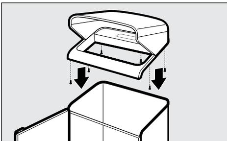
3. Attach hood to lid using the 6 packaged screws included.
