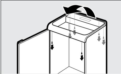
1. Detach lid – Remove the 6 screws on inside of container attaching lid to body. Rotate lid forward to release clips from container front.
