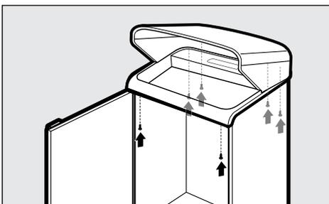
5. Reattach lid assembly to the base. NOTE: self-retaining washers at top of base may fall out while installing lid.
